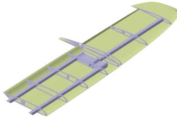
Fig. 4 Internal structure of the wing
