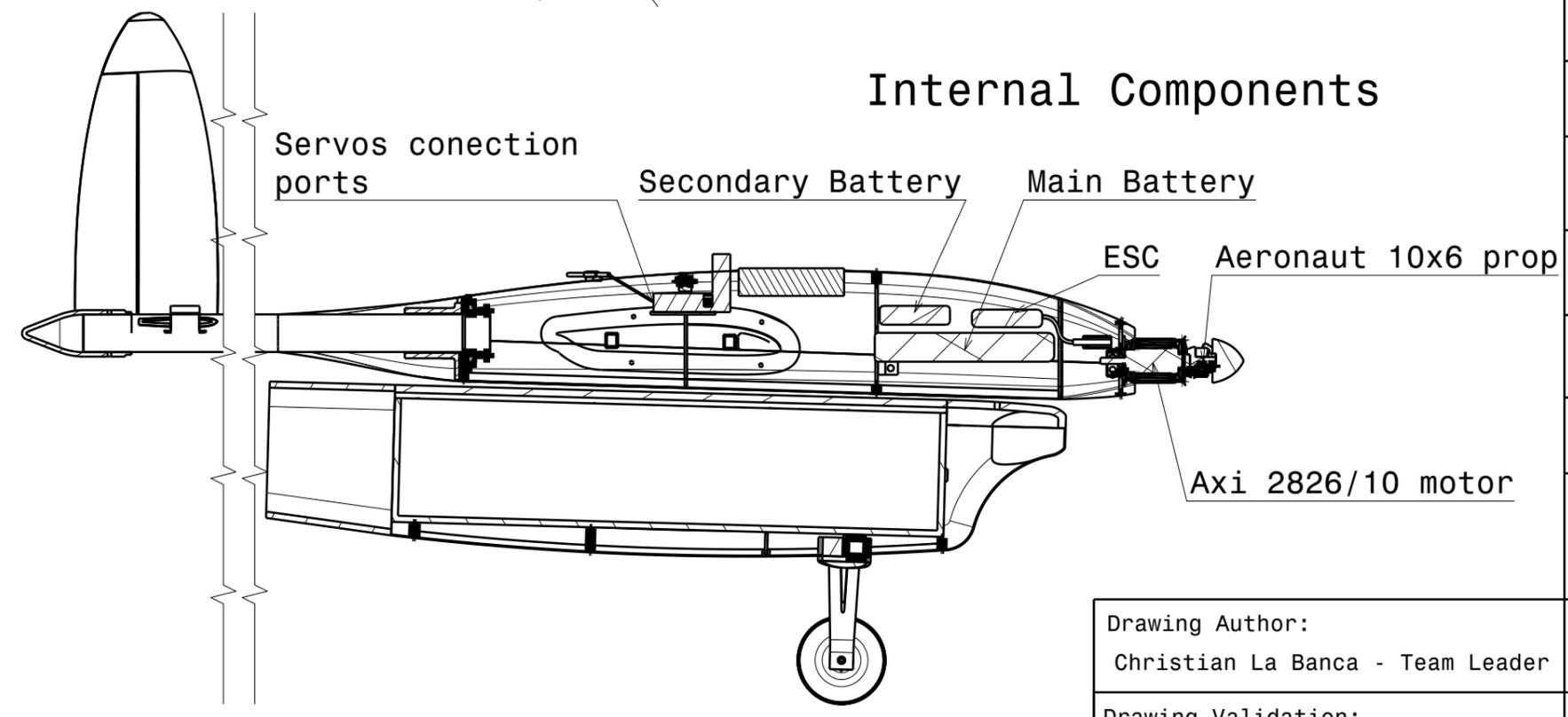
Section view. Internal components
