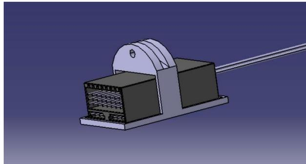
*Fig. 29 Receiver and its bracket assembly*
