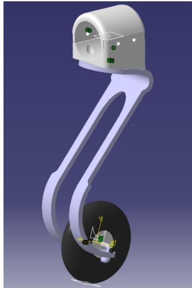
Fig. 27 CAD design of the rear landing gear
