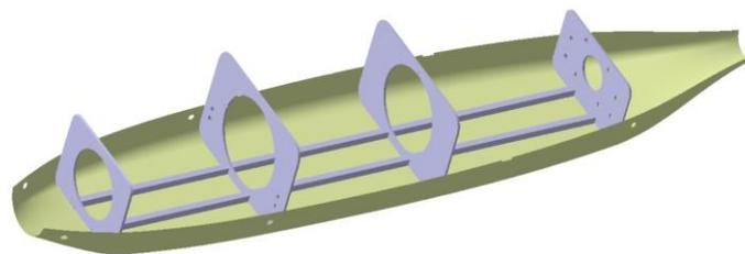
*Fig. 2 internal structure of the fuselage*
