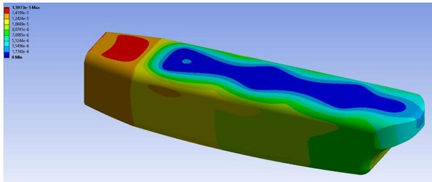
Fig. 40 Deformations with the weight on the landing gear.
