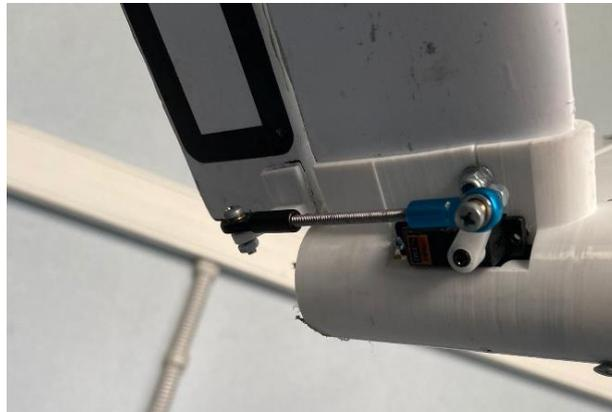
*Fig. 31 V-Tail mechanism assembly*
