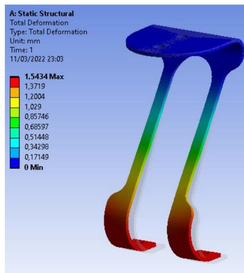
Fig. 28 Simulation of the rear landing gear
