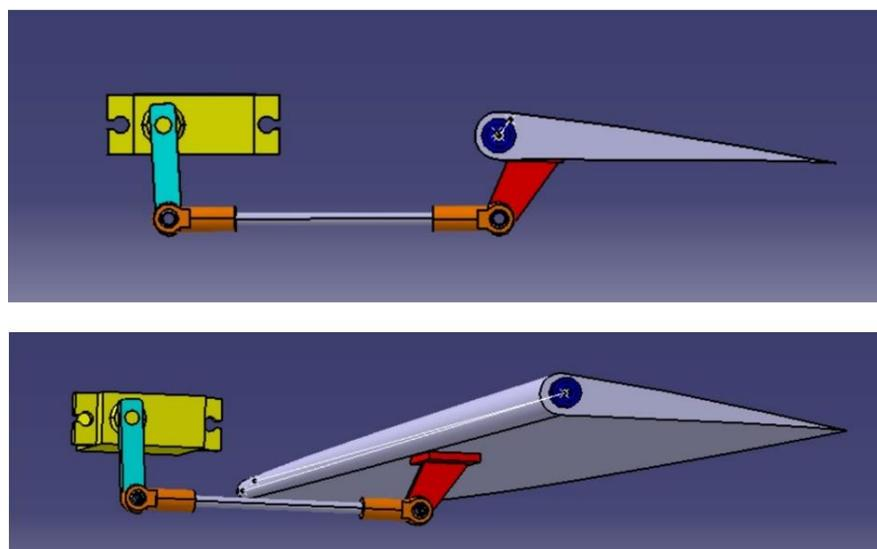
Fig. 30 Aileron Mechanism Assembly
