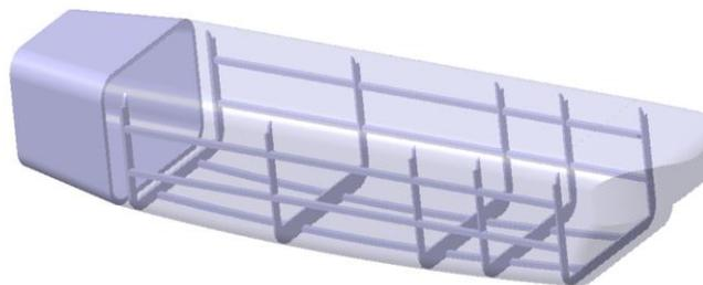
*Fig. 10 Internal structure of the cargo container*
