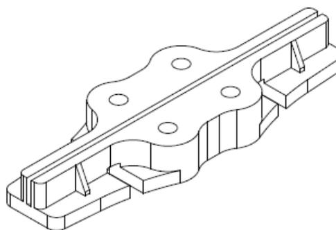
Fig. 25 Union of the main landing gear and cargo container
