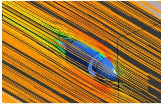
Fig. 22 3D streamlines of the propeller cone
