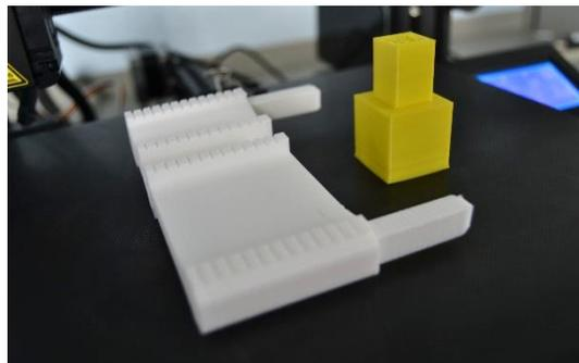
*Fig. 33 Left, PLA piece; right, TPU piece*
