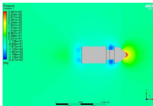
Fig. 21 Pressure field of the propeller cone
