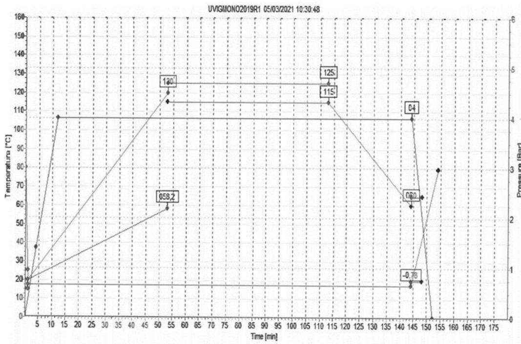
Fig. 38 Graph of the conditions during our autoclave cycles
