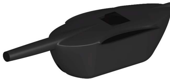
Fig. 4-10 Fuselage aerodynamic shape
