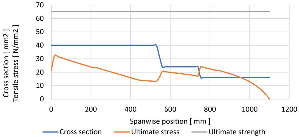
Figure 29: Lower spar cap stress
