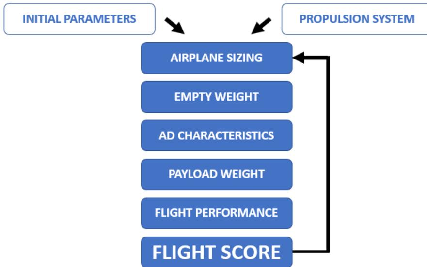
Figure 19: Aircraft shape optimization process
