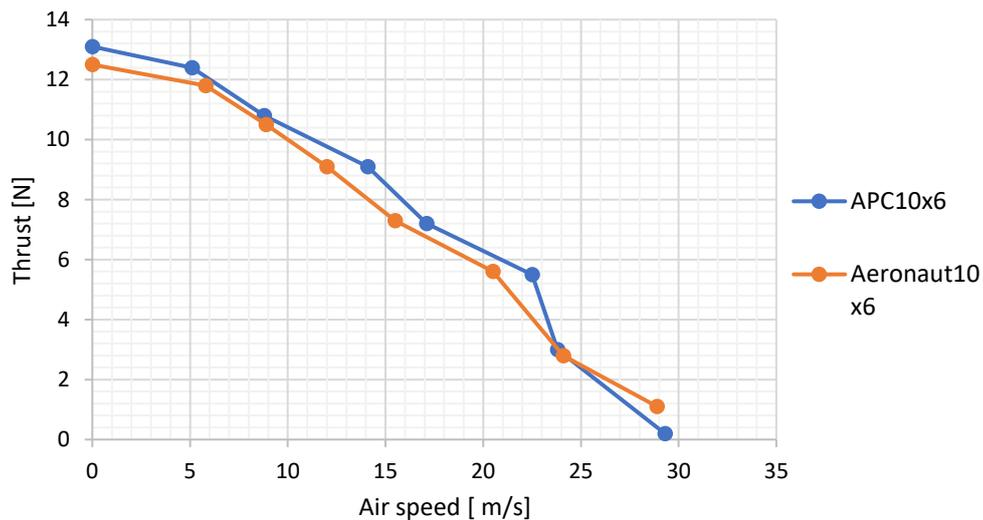
Figure 20: Propeller thrust diagram
