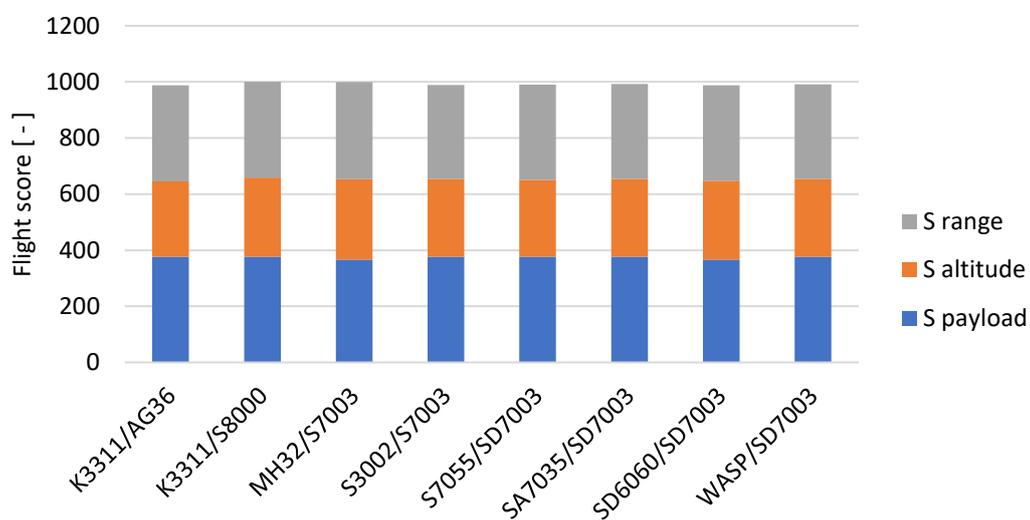
Figure 21: Airfoil influence - 3,5 kg payload, fixed wing
