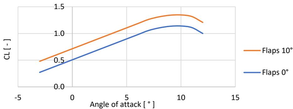
Figure 10: Airplane balanced lift line - middle CG
