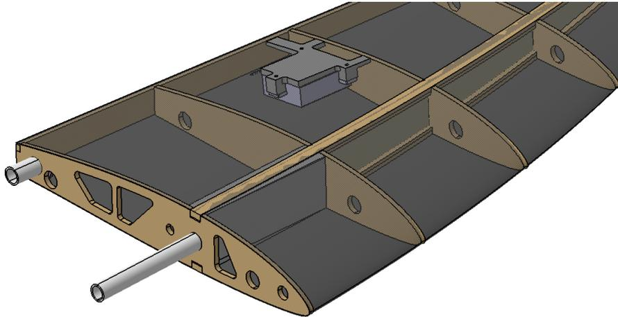
Figure 8: Wingtip structure
