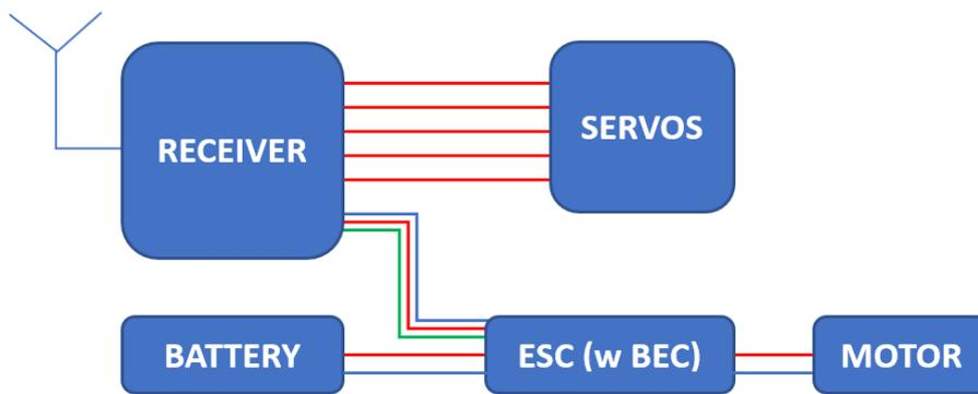
Figure 9: Propulsion electrical circuit scheme
