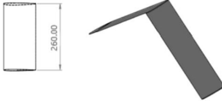
Figure 4.8 - Tail geometry, isometric and side view
