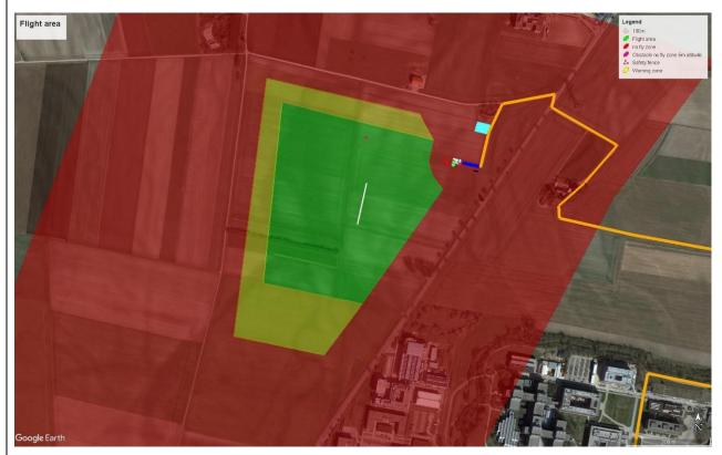
Figure 4: Flight Area: RED: No-Fly-Zone; BLUE: Flight area; GREEN: Landing field; BLACK: grass runway
