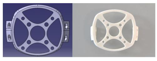
Fig. 18 Final motor mount. Left, CAD design; right, real assembly
