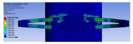
Fig. 24 Simulation of the main landing gear and cargo container
