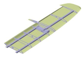
Fig. 4 Internal structure of the wing
