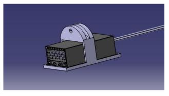
Fig. 29 Receiver and its bracket assembly
