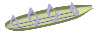
Fig. 2 internal structure of the fuselage
