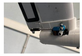
Fig. 31 V-Tail mechanism assembly
