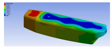
Fig. 40 Deformations with the weight on the landing gear.
