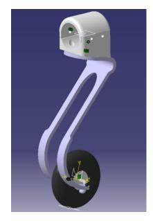
Fig. 27 CAD design of the rear landing gear
