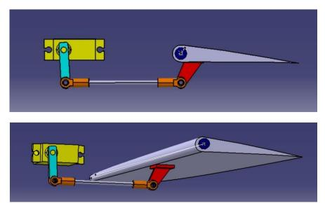
Fig. 30 Aileron Mechanism Assembly
