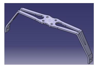
Fig. 23 CAD design of the main landing gear
