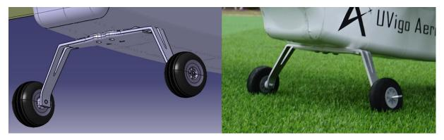
Fig. 26 Main landing gear. Left, CAD design; right, real configuration
