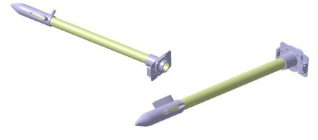
Fig. 9 Fuselage-empennage structure
