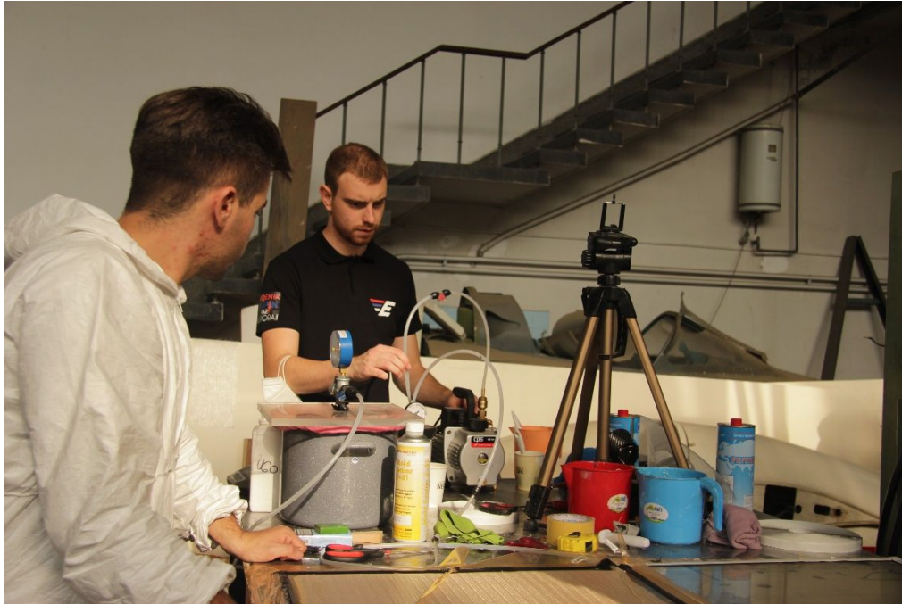
Figure 7.2 – Vacuum resin infusion process
