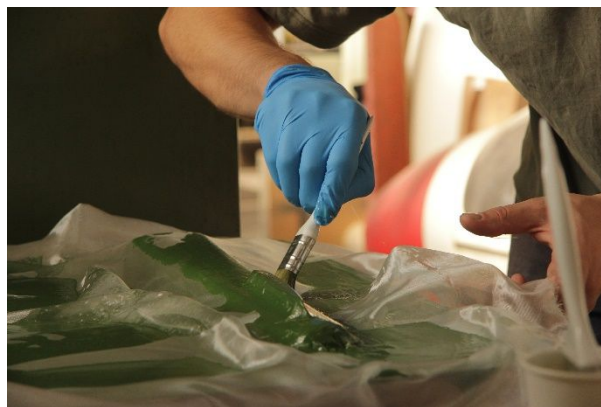
Figure 7.1 – Production of negative molds
