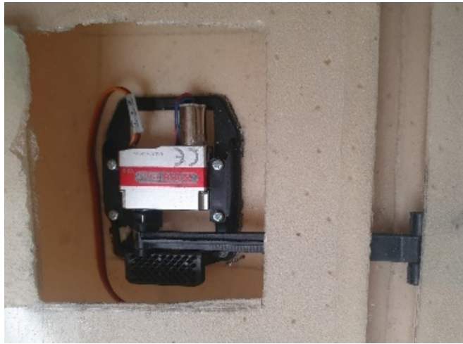
(a) aileron servo installation inside the wing
