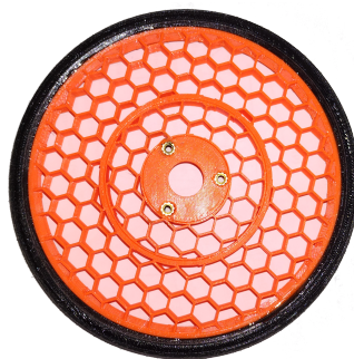
Figure 15: 3D printed main wheel
