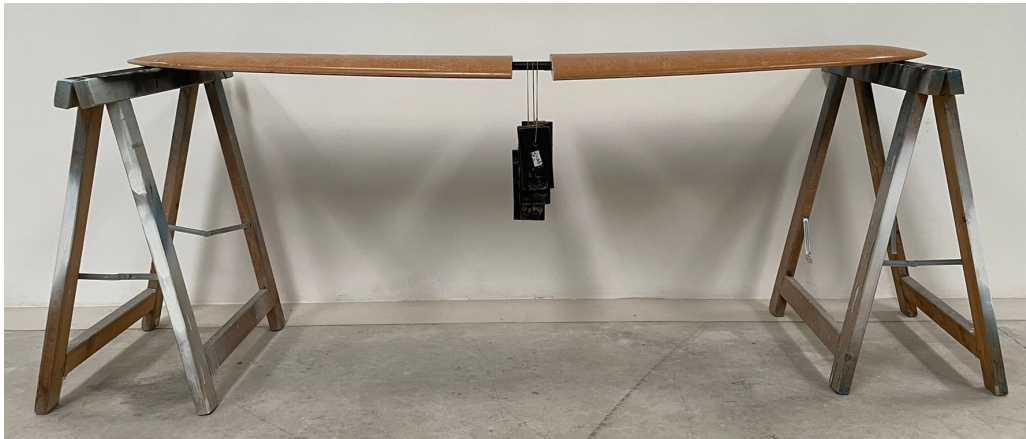
Figure 13: Wing undergoing load static test with 7500 g
