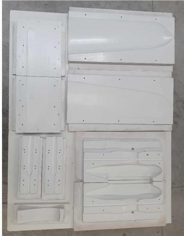
(b) the moulds after the surface treatment
