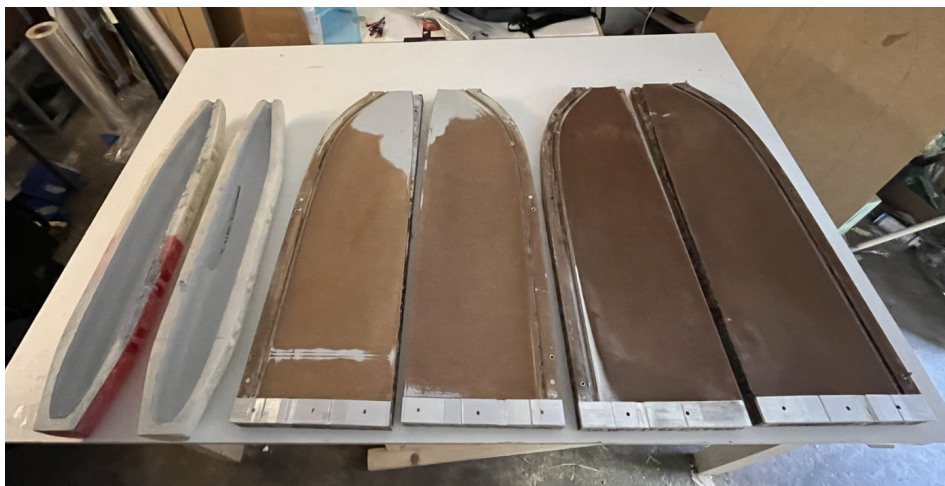
Figure 5.1: Molds of the fuselage on the left side and the wings on the right
