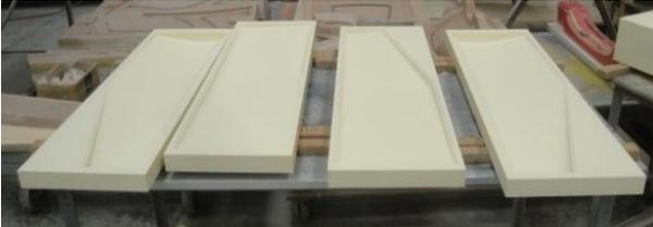
Figure 38 - Molds used to produce the composite components for the wing skin
