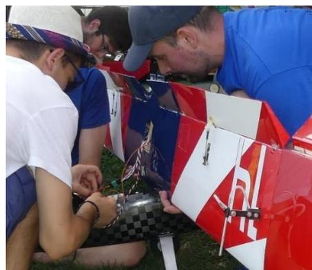
Figure 56 - Pitot tube mounted on Marcoplano (ACC2019)
