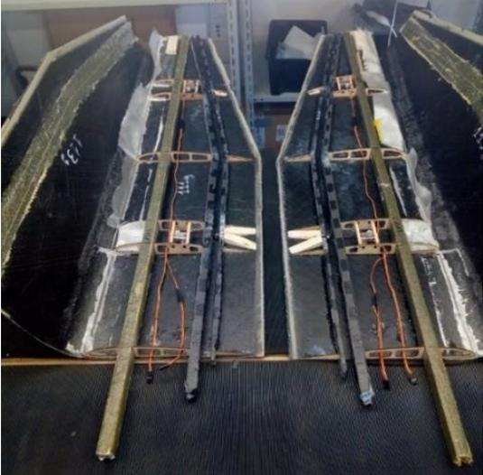
Figure 37 - Wing construction before closing the wing skins
