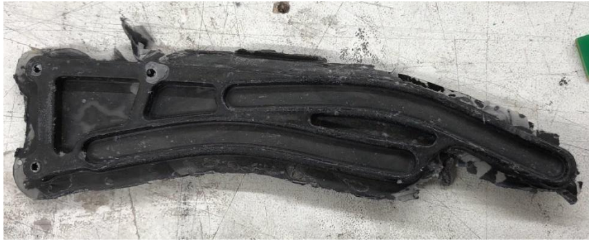
Figure 7-4 The centre rail directly after demolding
