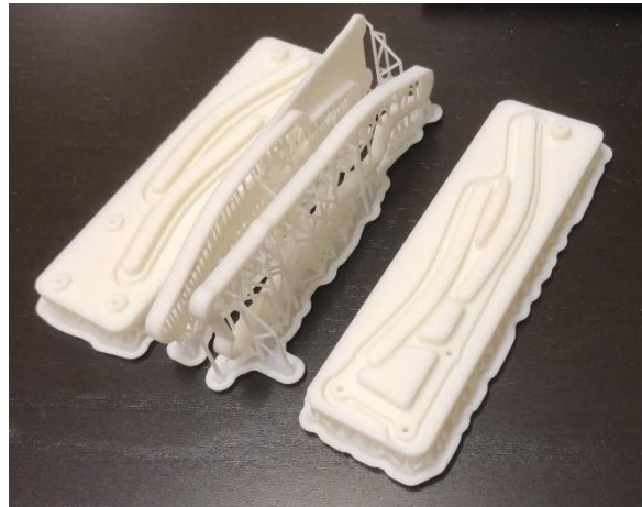
Figure 7-3 The resin printed molds for the center rail
