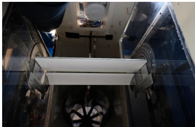
Figure 6-4 The model installed in the wind tunnel.
