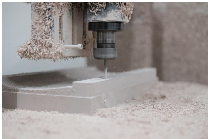
Figure 7-2 The milling machine during the production of one of the molds
