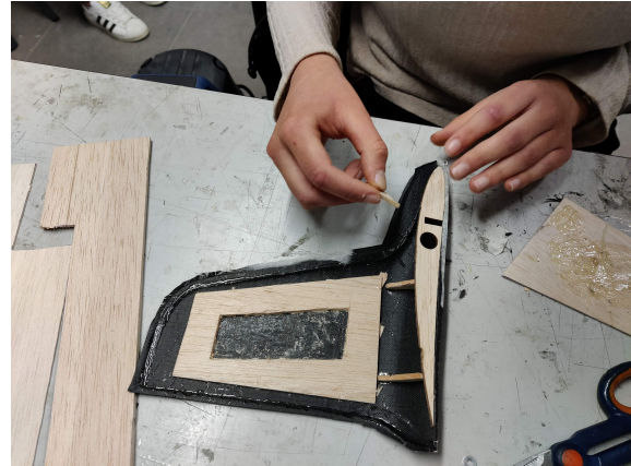
Figure 22: Internal structure of the winglet
