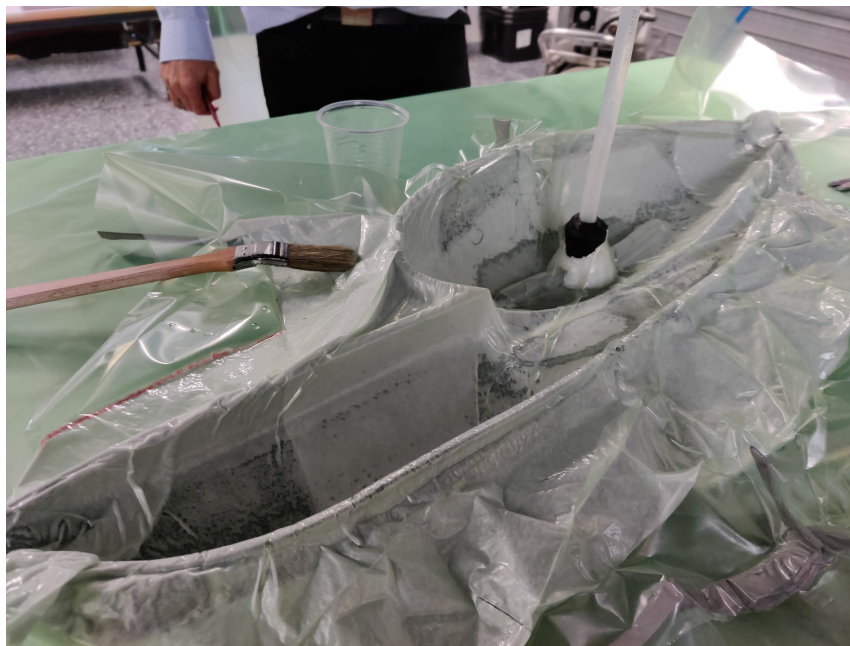
Figure 23: Vacuum lamination of the cargo bay
