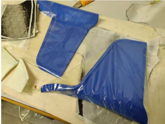
Figure 21: 3D printed winglet molds
