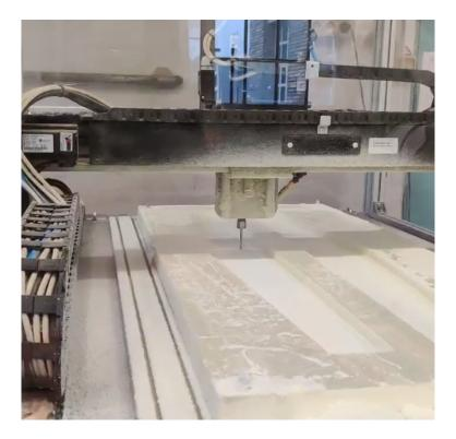
Figure 16: CNC working on the fuselage mould
