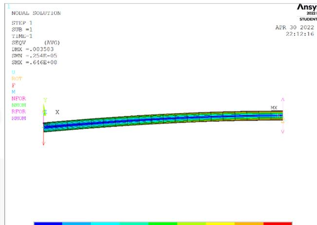
Figure 35. Von-Mises stress in a carbon fiber spar [Pa].
