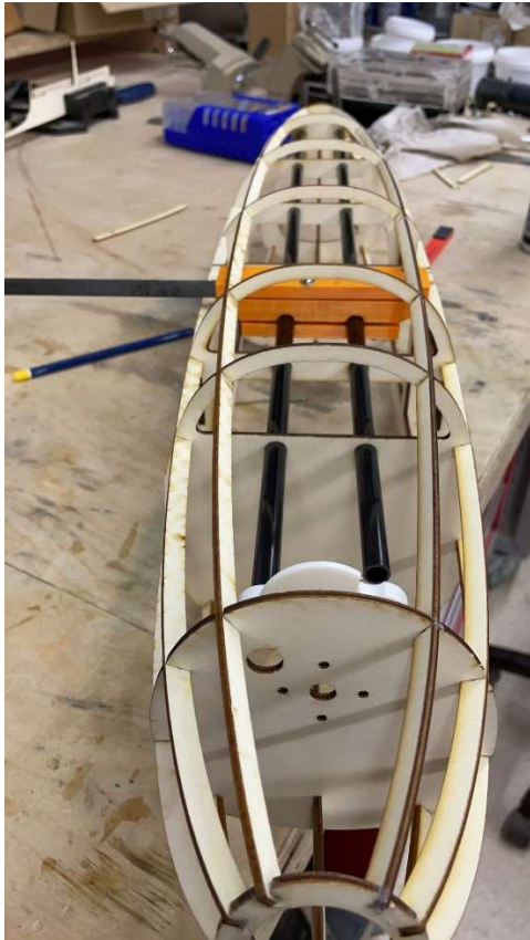
Figure 2: Fuselage structure made out of two CFRP Tubes and wooden frames and stringer
