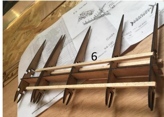
The different components of the structure are kept in contact using notches and epoxy adhesive.
