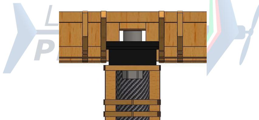
The vertical tail contains almost the same elements of the horizontal tail with the exception of a main composite spar instead of a wood one.
