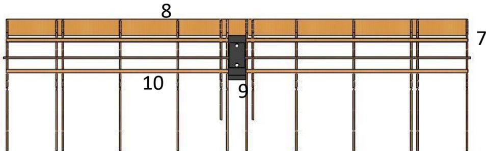
There are one main spar (7) and four other stiffening and stabilizing longitudinal elements (10). In addition, the leading-edge element (8) provides more stability to the ribs. The number 9 is a 3D printed connection plate that we have used to join the horizontal to the vertical surface by means of two M4 screws, as shown in the following image:
