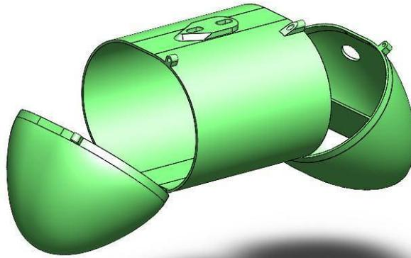
These parts are made by 3D printing of plastic, reinforced with Kevlar fibers. The choice of Kevlar instead of Carbon fibers has been made because we needed the bay shell to be “transparent” to the electro-magnetic radiation. The fairings are connected to the central part with four hinges (two for each side) that allow the relative rotation.
