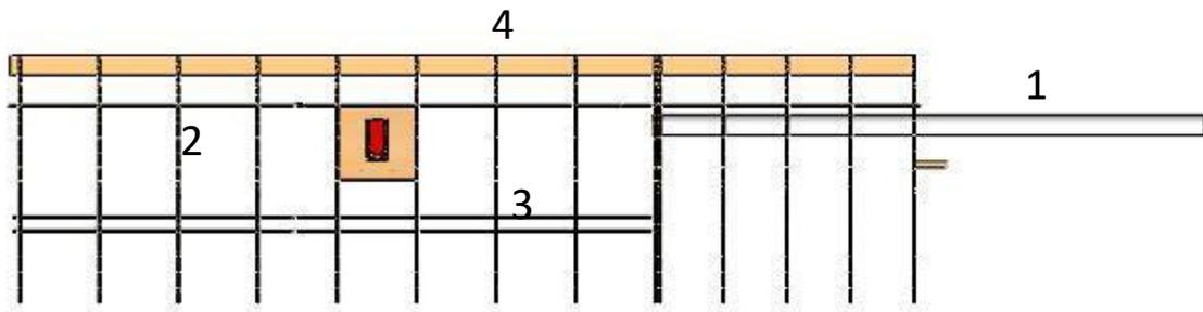
The transversal elements (5) consist of wood ribs. We have chosen two different spacings for the inboard and the outboard half-wing, with a “separation” section in correspondence of the aileron breaking section, where we have decided to place two ribs very close to each other.
