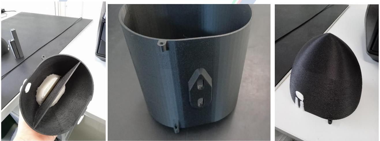
The whole bay assembly is attached to the central joint described in [section 5.2](#) with the same two M6 bolts that pass through the fuselage tube. For this reason, a region of increased thickness is present in correspondence of the joint location. A horizontal “shelf” has been designed to accommodate the servos battery and the receiver in the back of the bay. A circular hole realized in the top of the rear fairing allows the passage of the wires.
