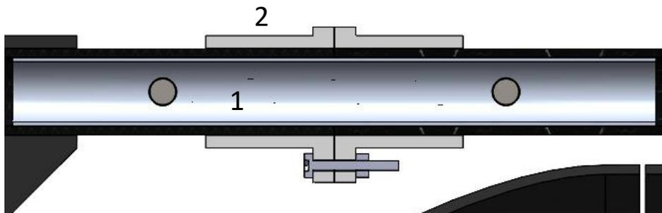
The internal tube is fastened to the two sections of fuselage by using M6 bolts, while the external parts are mounted with interference on the carbon tubes and then connected by means of M3 screws. This type of joint has proved to be very effective in transferring the driving force of the engine to the rest of the model and to inhibit relative rotations between the two sections of fuselage.
