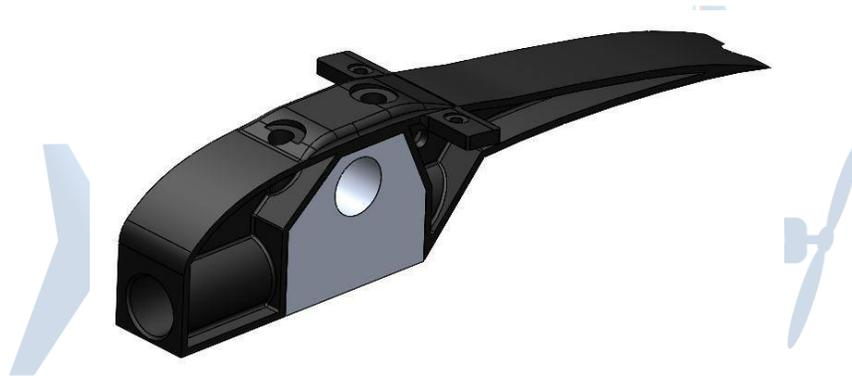
The central joint also provides the point of attachment of the two half-wings to the rest of the model, by means of two M4 screws that go right into the corresponding drive-in nuts placed inside the structure of the wing.
