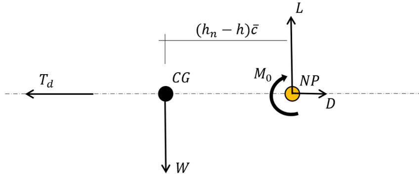
The total lift and drag,  $L$  and  $D$ , are applied in  $NP$  and  $M_0$  is the zero-lift total aerodynamic moment calculated with respect to  $NP$ :
