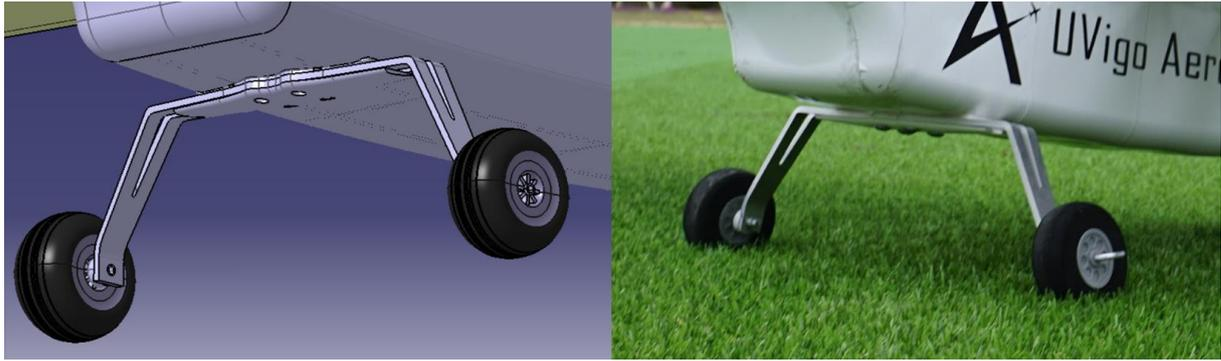
Fig. 26 Main landing gear. Left, CAD design; right, real configuration
