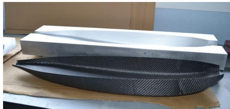
Fig. 35 Final result of our carbon fiber parts
