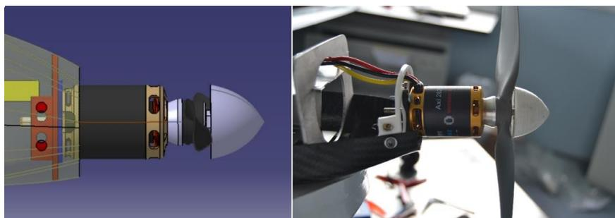
*Fig. 19 Main motor assembly. Left, CAD design; right, real assembly.*
