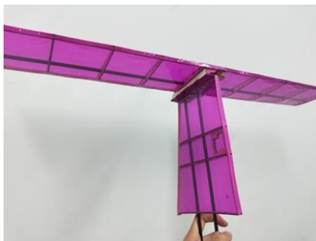
Figure 3.3 Wooden T-tail without rudder surface
