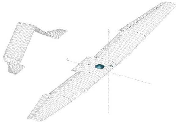
Figure 27 – Panel distribution analyzed in XFLR5
