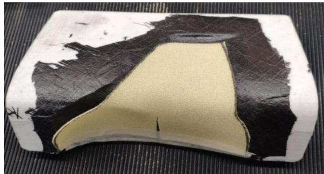
Figure 41 - Laminating sandwich structure on the winglet mould
