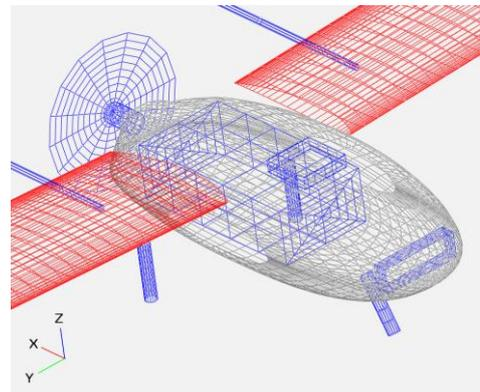
Figure 21 - Position of elements inside the fuselage
