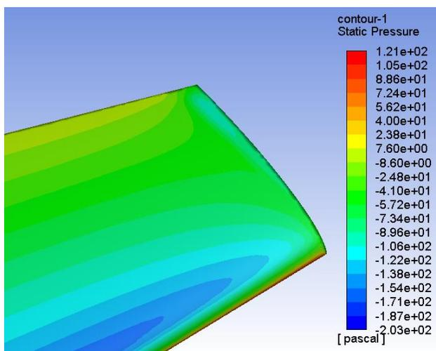
Figure 15 – Static relative pressure without winglet
