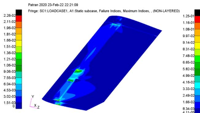
Figure 47 - Maximum failure indices
