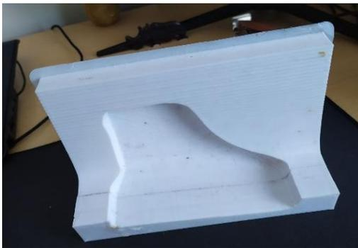
Figure 40 - Mould of winglets produced by 3D printing technology
