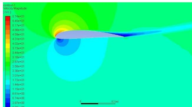
Figure 6 – Velocity magnitude at  $\alpha = 15^\circ$
