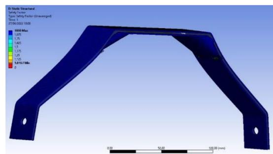
Figure 52 – Main gear, safety factor
