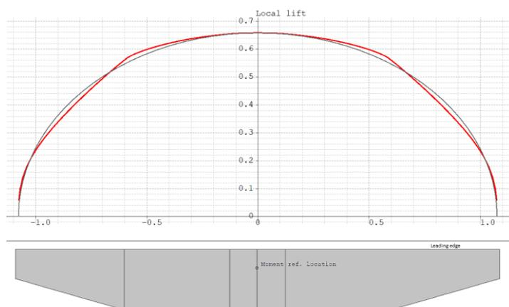
Figure 13 - Wing's lift distribution compared with the ideal one
