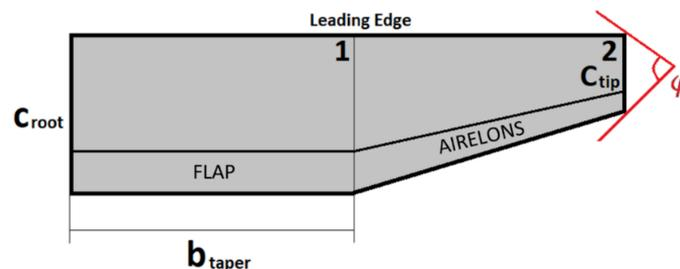
Figure 11 - Wing planform's main geometry properties
