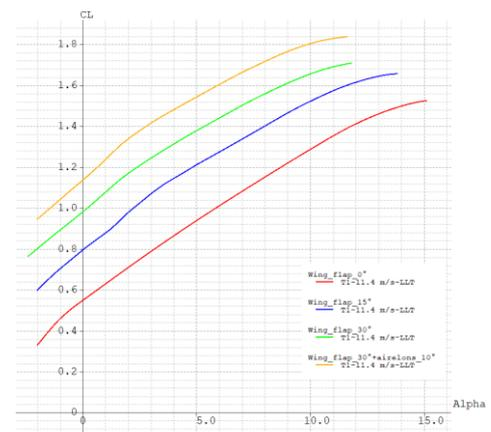
Figure 14 - Wing  $C_L$ - $\alpha$  at different flap deflections
