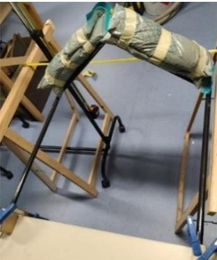
Figure 49 - Loading the tailplane assembly
