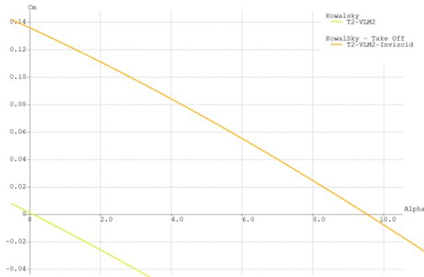
Figure 26 –  $C_M$  vs  $\alpha$  trimmed in cruise and take-off conditions
