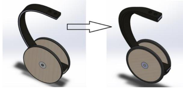
Figure 24 - Evolution of the front undercarriage design
