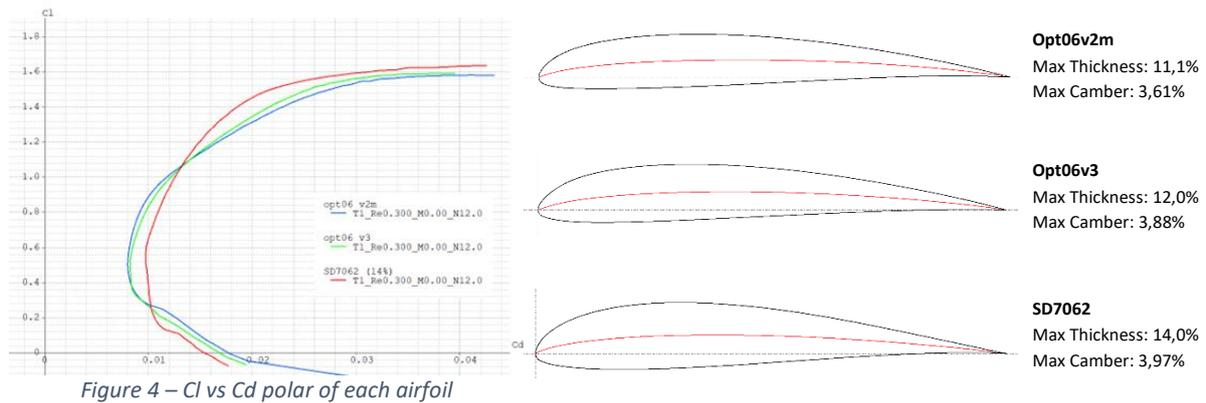
Figure 4 –  $C_L$  vs  $C_D$  polar of each airfoil
