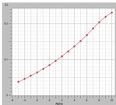
Figure 22 - Fuselage  $C_L$  vs  $\alpha$
