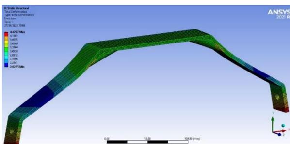
Figure 51 – Main gear, total deformation
