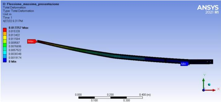
Figure 35 - Maximum total deformation from FEM analysis (left wing)
