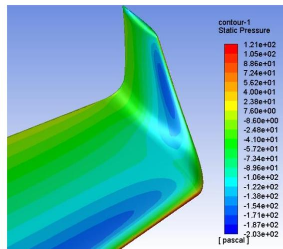
Figure 16 - Static relative pressure with winglet
