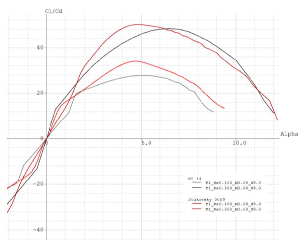
Figure 19 - Tail's airfoils efficiency vs alpha comparison at  $Re=1e5$  and  $Re=3e5$
