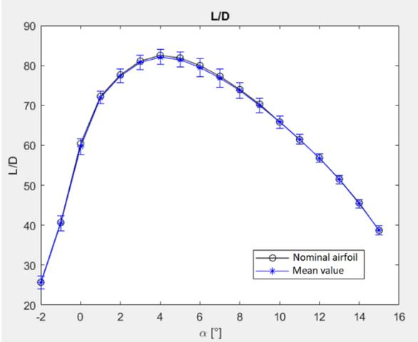
Figure 9 - Airfoil efficiency vs alpha
