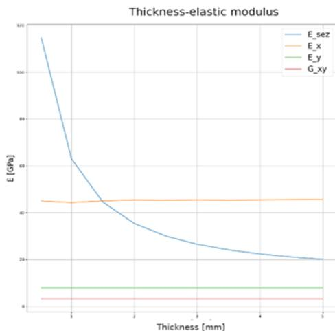
Figure 33 - Results of the elastic modulus obtained with Eq. 5.1.1 and Eq. 5.1.2
