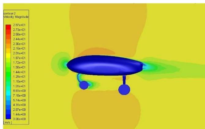
Figure 23 - Mid-plane velocity magnitude at  $\alpha = 0^\circ$
