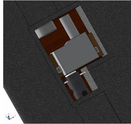
Figure 45 – Servo installation inside the tailplane
