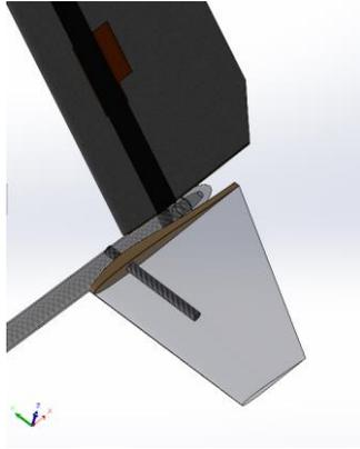
Figure 44 - Pitch fin structure
