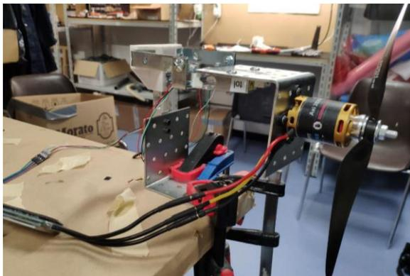
Figure 55 – Propeller test bench
