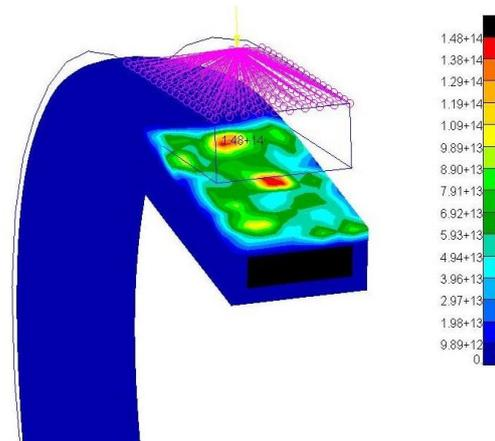
Figure 54 – Nose gear, max strenght ratios
