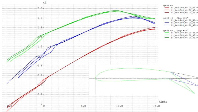
Figure 10 -  $C_l$  vs alpha at different flap deflections and Reynolds Number
