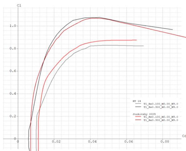
Figure 18 - Tail's airfoils  $C_l$  vs  $C_d$  comparison at  $Re=1e5$  and  $Re=3e5$
