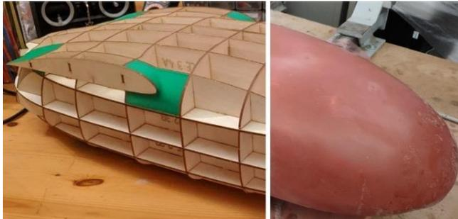
Figure 42 - Handmade master during and after construction
