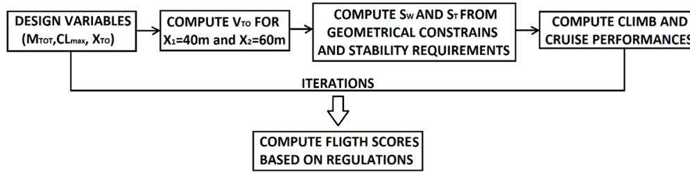
Figure 2 - Flow chart of preliminary design algorithm
