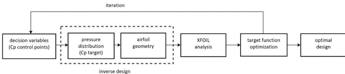
Figure 3 - Flow chart of wing airfoil optimization algorithm
