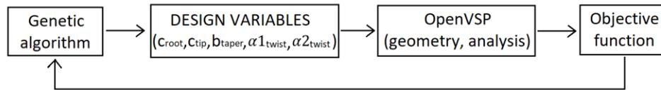
Figure 12 - Flow chart of wing's optimization algorithm
