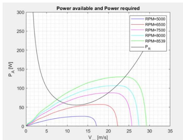
Figure 29 - Power available and Power required in function of V and RPM
