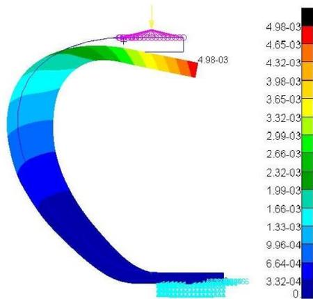
Figure 53 – Nose gear, translation displacements
