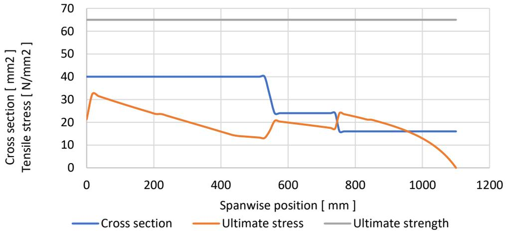
Figure 29: Lower spar cap stress
