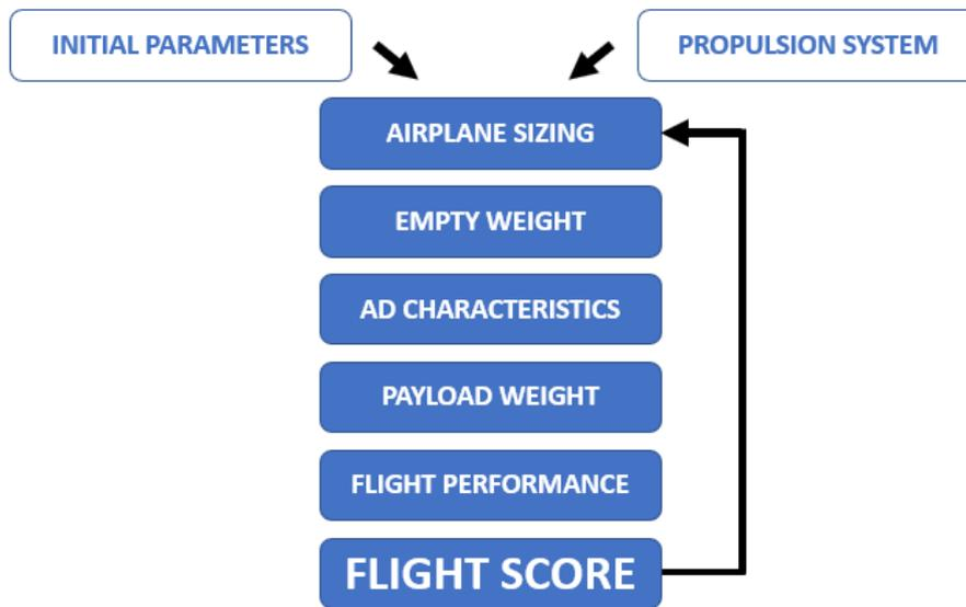
Figure 19: Aircraft shape optimization process
