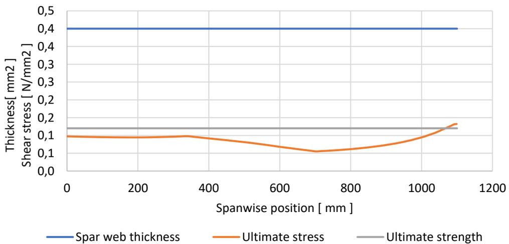
Figure 30: Spar web shear stress
