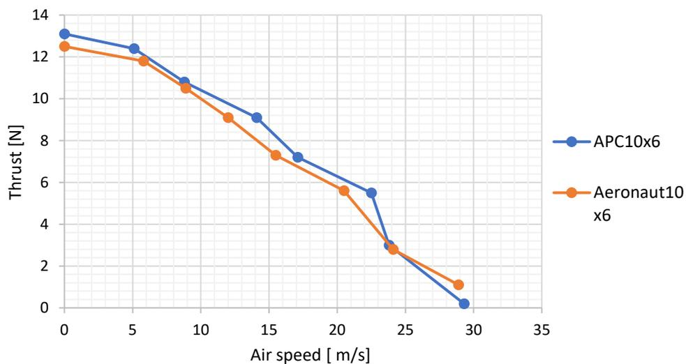
Figure 20: Propeller thrust diagram
