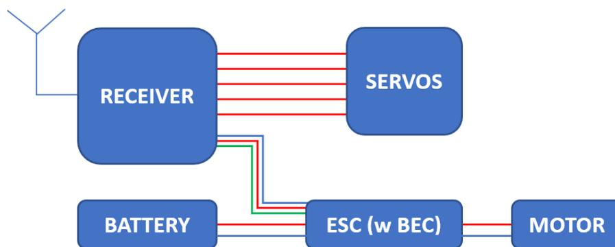
Figure 9: Propulsion electrical circuit scheme
