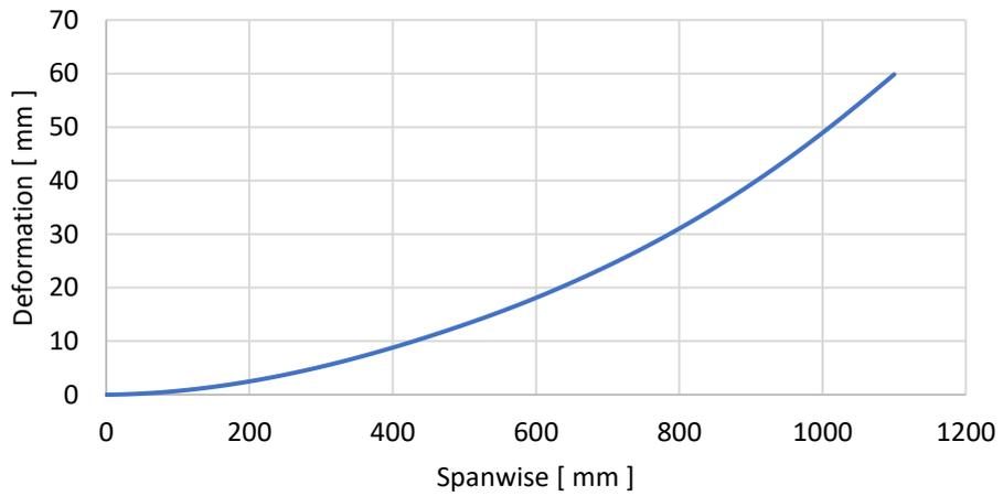
Figure 31: Wing bending deformation
