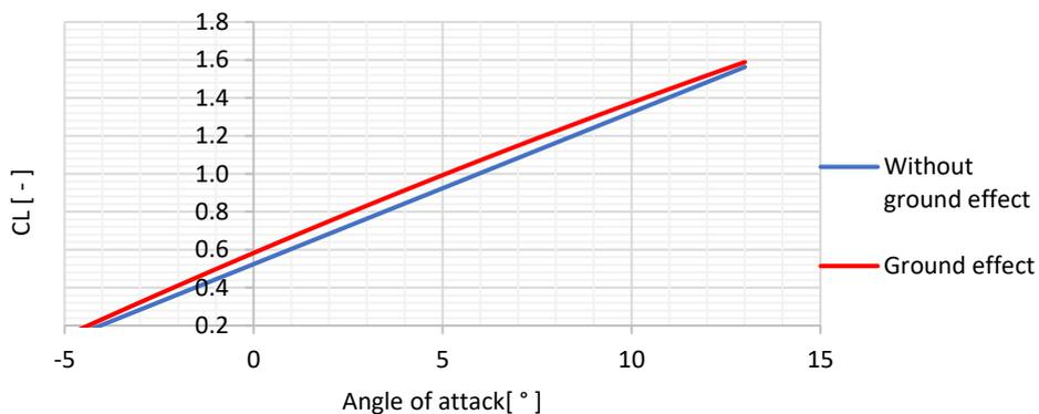
Figure 11: Balanced lift line - middle CG, Flaps 25°
