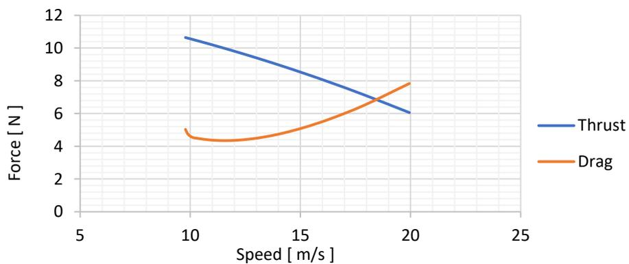
Figure 18: Thrust/drag diagram
