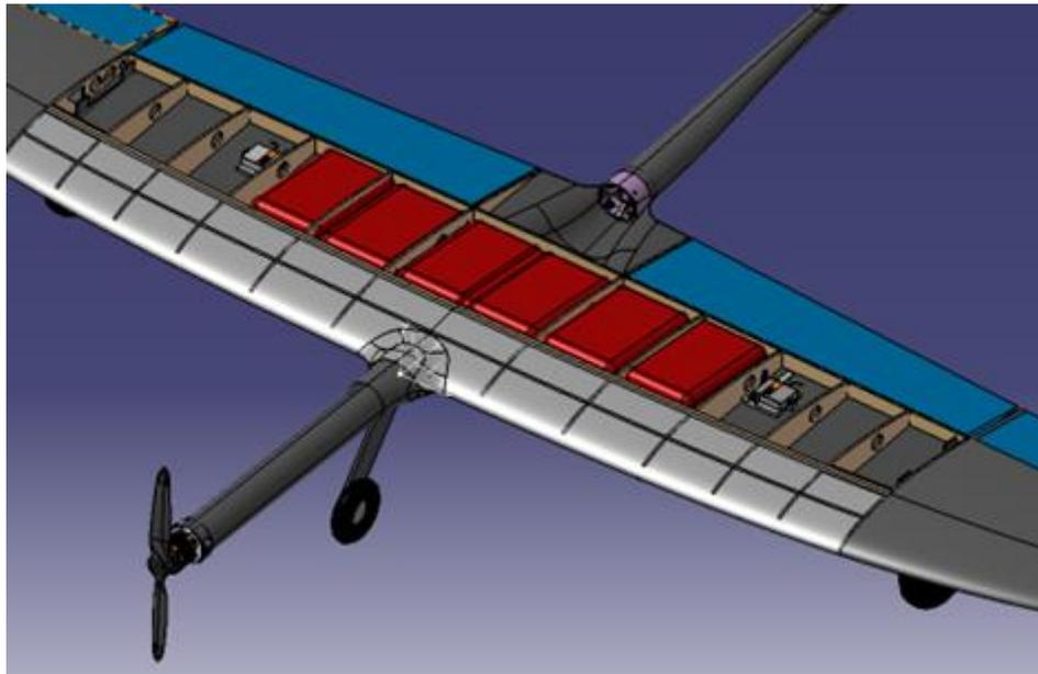
Figure 6: Storage of cargo in wing
