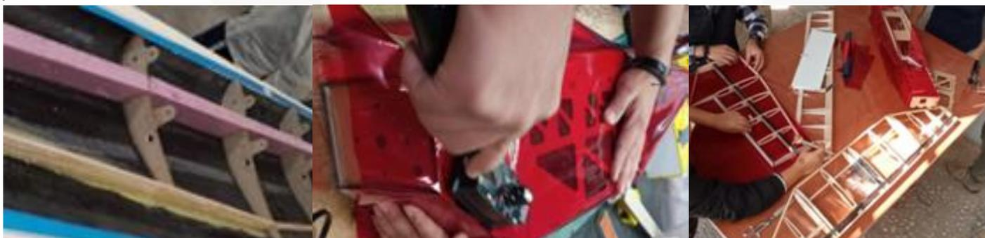
Figure 37. U-FLY's past manufacture process. From left to right: a 4m span wing of carbon fiber; recovering a fuselage with Monokote; conventional tail empennage assembly.
