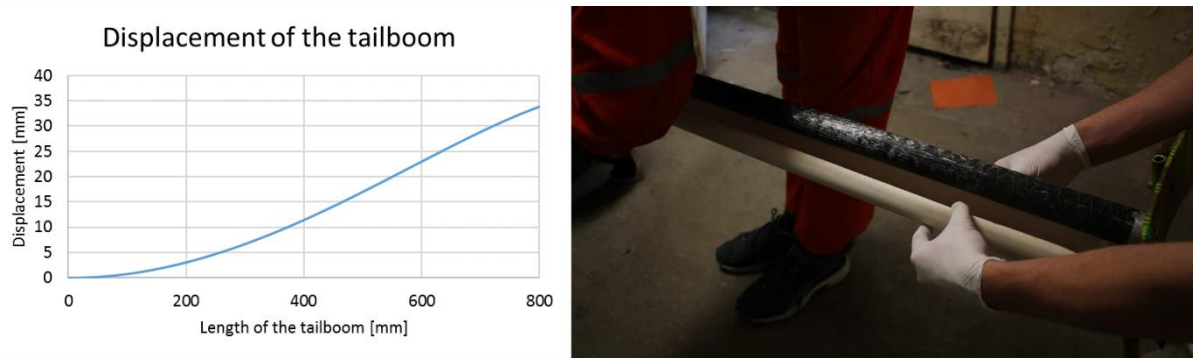
Figure 23 Tail boom displacement chart and measurement method
